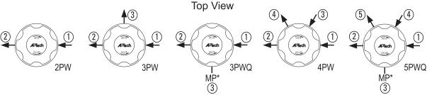
All dimensions in inches. Metric dimensions (mm) are for reference only. MP=Monitor port, first stage outlet pressure (second stage inlet pressure). Numbers at each port note order for specifying fitting type.
